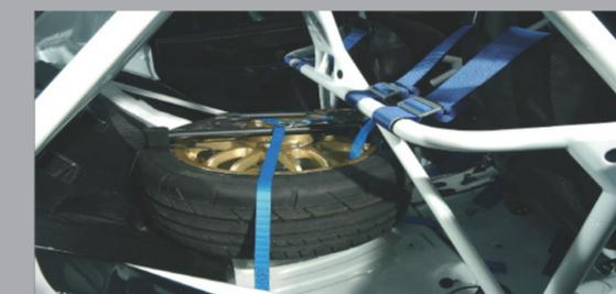
The 2006 Group N features a new aerodynamic package and a revised interior with a new roll cage, enabling two spare wheels to be fitted inside the car.
